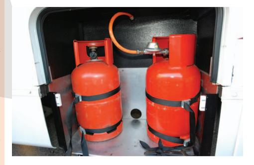
All cylinders must be adequately secured against movement of the ship with the supply shut off at the cylinders during the voyage. Leaking and inadequately secured or connected cylinders will be refused shipment. Any gas cylinders to be carried must be declared at the time of booking. Partially full or empty cylinders will be treated as if they are full.
