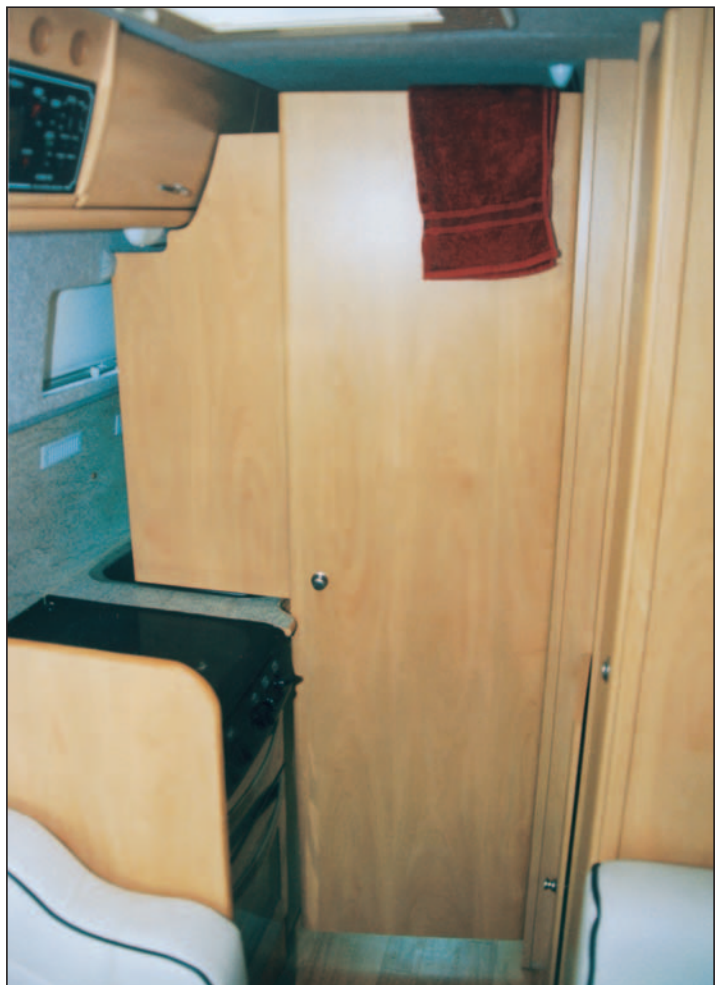
This is a good idea. Bi-fold washroom door opens out to create a dressing room from of the rear portion of the central aisle.
