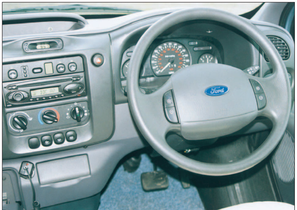
Ford cab is well laid out. Buttons on steering wheel allow manual gearchanging if desired. I opted for fully automatic and let the electronics take the strain.
