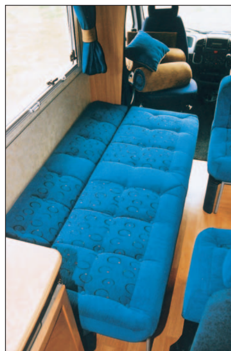
Squabs slide and backrests drop in to form a generous, offside single.
