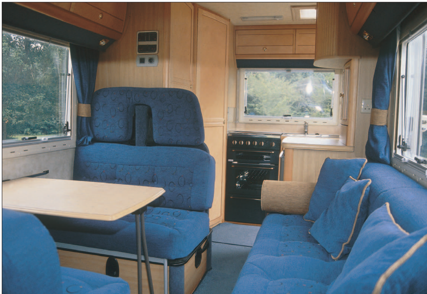
Dinette (with forward-facing belted seats for two) opposite longitudinal settee, makes a practical four-berth layout. The kitchen and washroom live comfortably in the rear.
