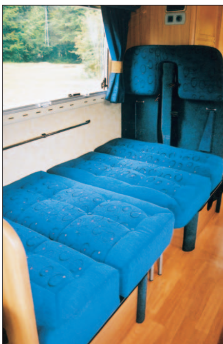
Slide the sofa base forwards to make the nearside berth. With two single beds in use there's a very narrow aisle in between.
