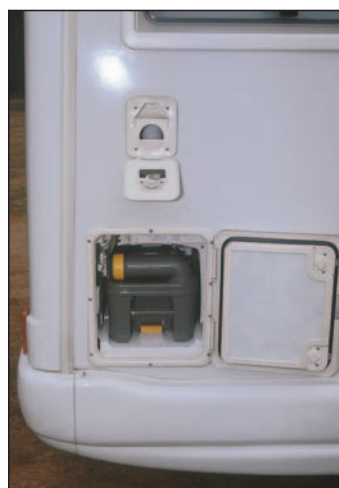
The toilet cassette is easily accessed. Above is the flushing tank filler.
