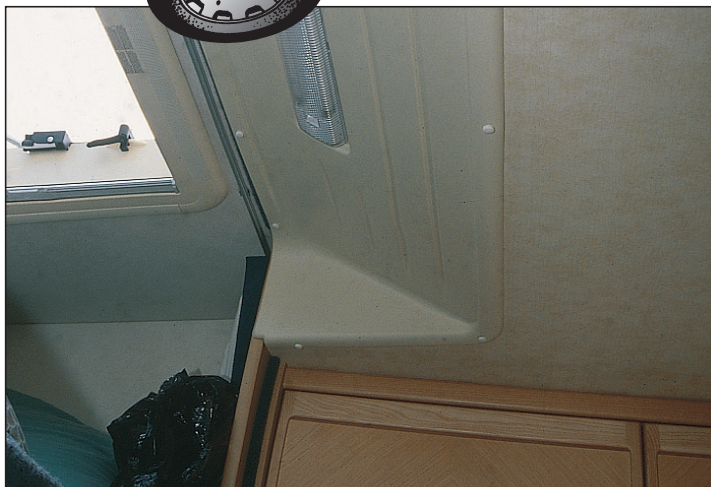
This is the light for the overcab bed. The angled roof section with light plastic liner helps make this space user-friendly.
