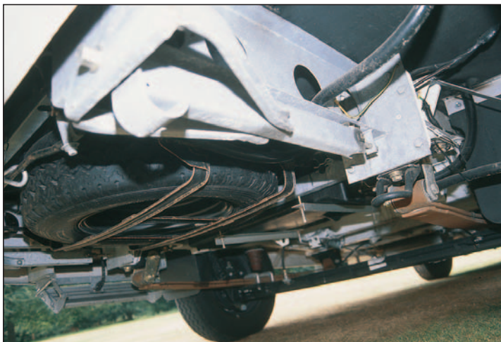
Spare wheel is relatively easily accessible. The rear steadies are an optional extra.
