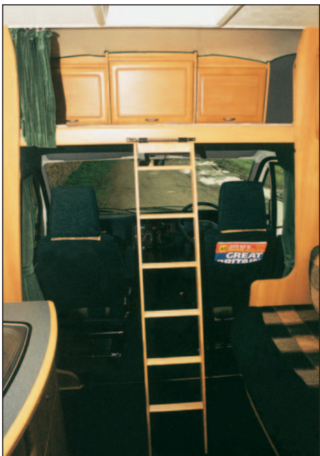
Overcab bed is suitable for occasional use, or for a child. There's no storage provision for the mattress or ladder.
