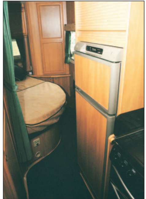
The 135-litre fridge/freezer decides for itself between 12V, 230V or gas power.
