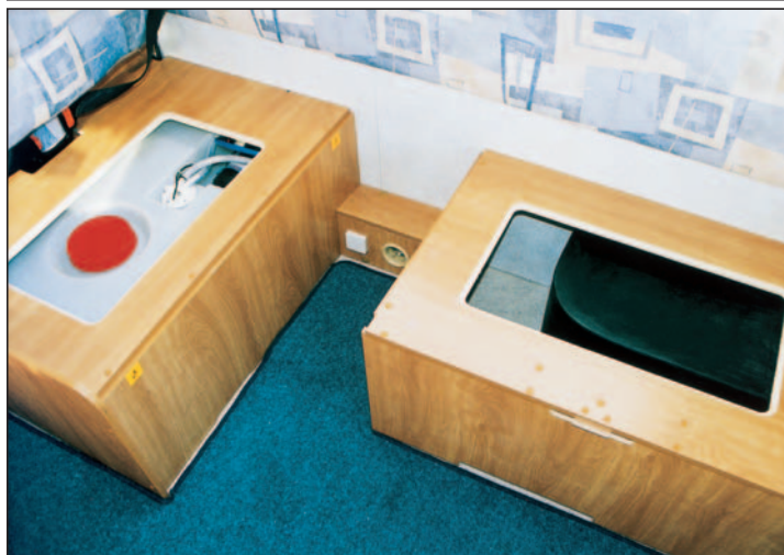
Underseat space is mostly full of fresh water tank (thankfully in view of on-test temperatures) and externally accessed gas locker.
