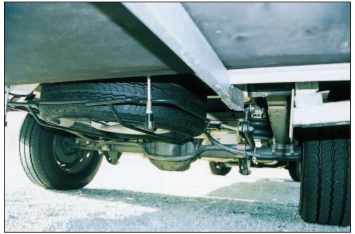
Worm's eye view shows inaccessible spare wheel cradle, air bag suspension assisters, and part of the galvanised subframe that runs full length and width between the Merc's chassis rails and the floor decking.
