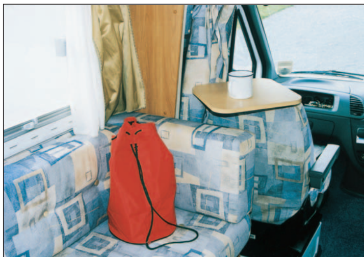
Southdowns' Sailers arrive complete with this natty coffee table. It locates in the headrest mounting holes.
