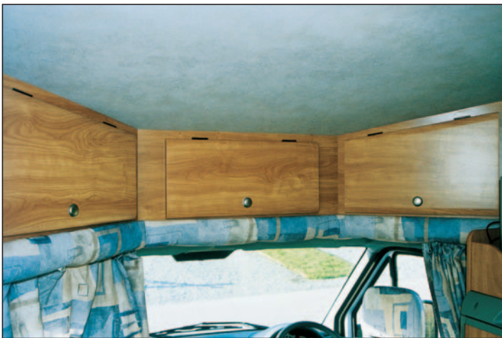
Cab roof is cut away with a trio of angled lockers placed around the edges.
