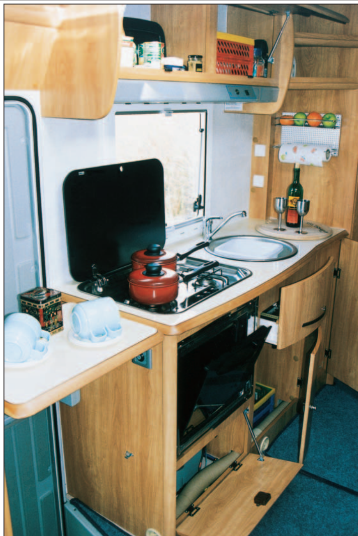
The Brit-friendly kitchen, with worktop extended across doorway. The blown-air heater outlet on the end panel counteracts the draught from the gas dropout vent in the footwell.
