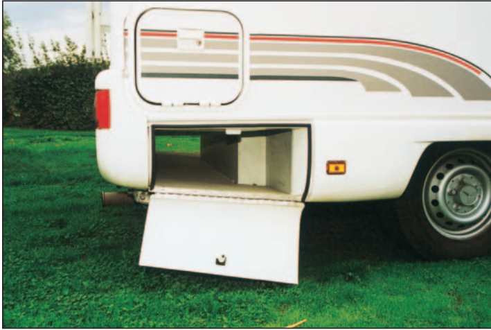
Underfloor locker has bottom-hinged doors on either side and is ideal for long objects such as skis or awning poles.
