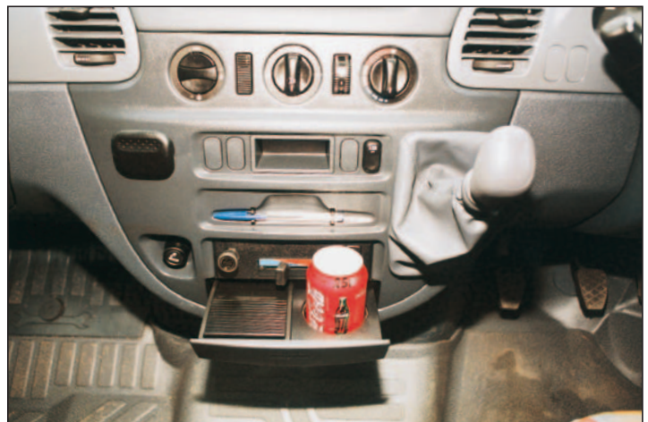
Latest Mercs have excellent fascia-mounted gearshift. See also neat drink holder and (behind the can) rear passenger heating controls.
