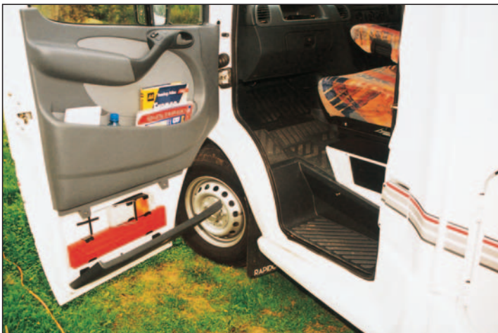
Both cab doors have useful storage pockets and below these are 'secret' panels - passenger side hides warning triangle and lamp.
