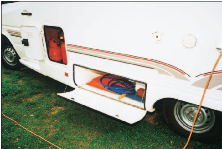
Nearside skirt incorporates moulded locker, but weight of contents made skirt panel bow outwards. Further forward is gas locker.
