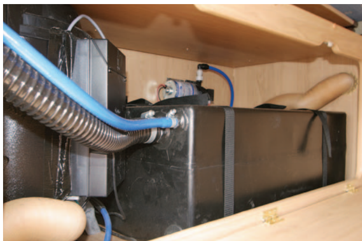
The Truma Combi boiler and fresh water tank are located right in the tail end of the underbed store.
