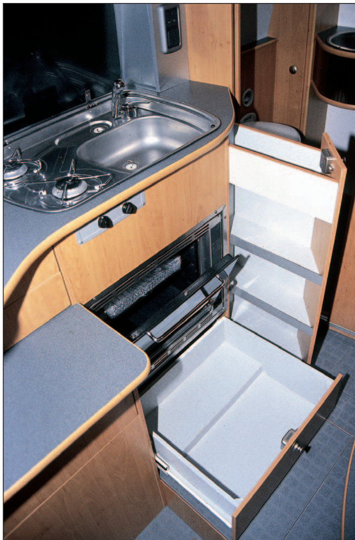
Combined two-burner hob and sink proved to be a space-saving design. Kitchen storage ranges from cutlery and towel drawers to something suitable for pots and pans. An innovative, slide-out unit will take all the jars, cans and bottles you might need.
