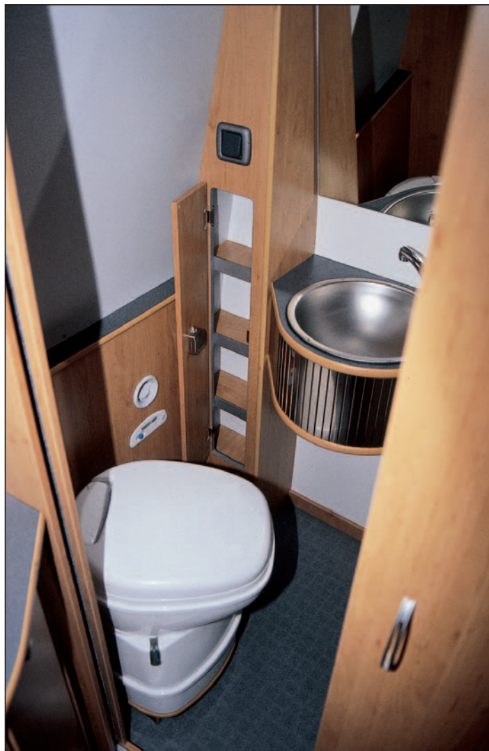
Across-the-rear bathroom has an electric-flush loo and a shaving-friendly basin and mirror.
