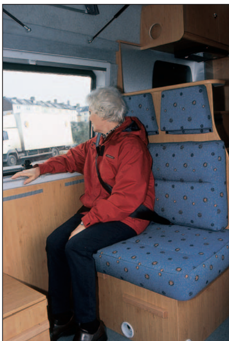
Rear seat passengers are afforded leg room by the removal of the side cushion. There is one three-point belt and one lap belt.
