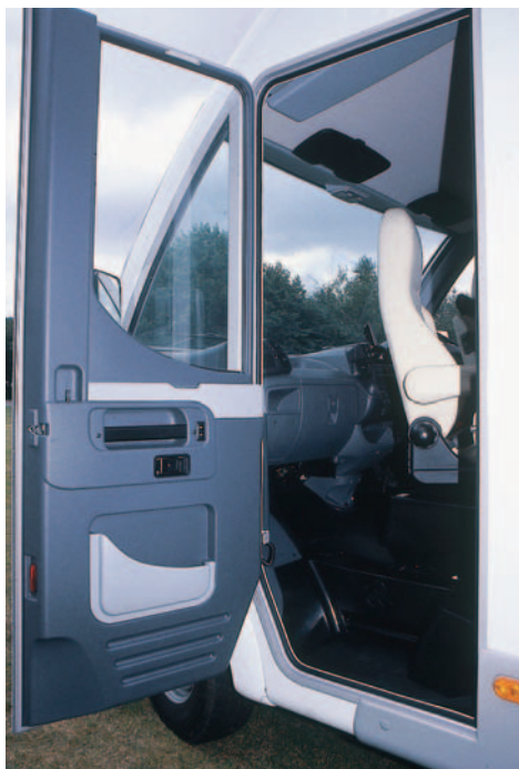
Continental handing of the body means the single cab door is on the UK nearside.
