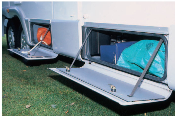
All around the skirts are access hatches that allow you to get at the between floor storage.
