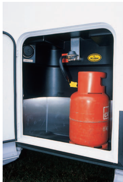
The water filler is incorporated into the top left of the gas locker.
