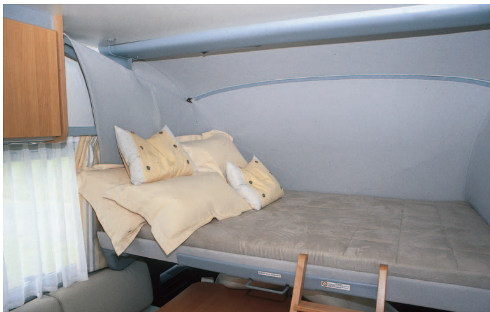
With the Aguti pilot seats folded, the overcab bed lowers to a height that makes it easy to step straight up into the bed from the lounge seating.
