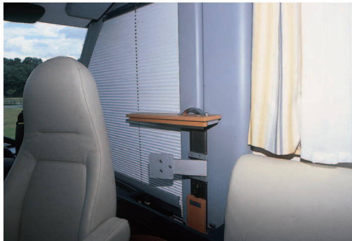
You can screw a flat screen television to the aluminium bracket that pops up in the cab. It can be easily adjusted to obtain an optimum viewing angle.
