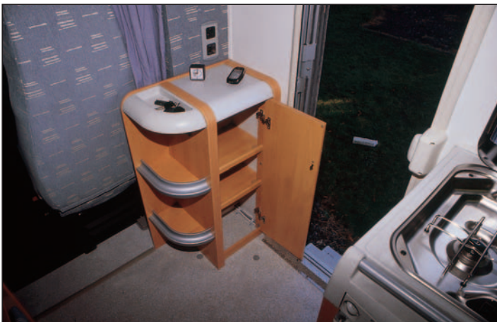
The fitting of an oven robs the kitchen of a cupboard, but this unit is just the other side of the caravan door. The top has sockets for TV.
