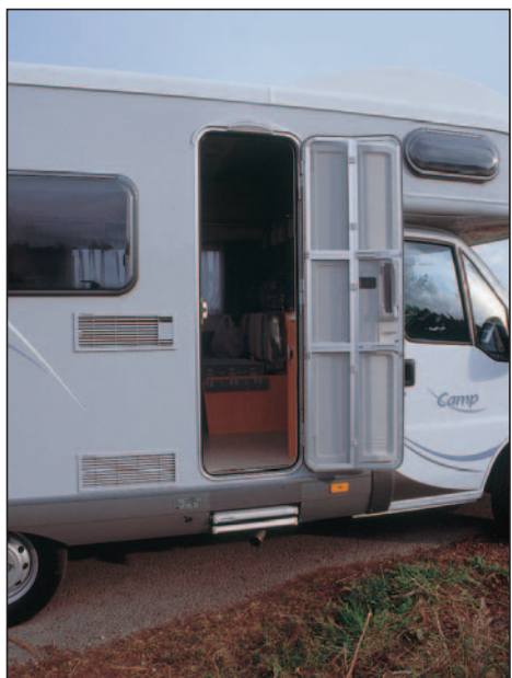
UK offside caravan door opens to reveal a folding flyscreen. The door stays clear of the fridge vents when open. Neatly integrated porch light can be seen at the top.
