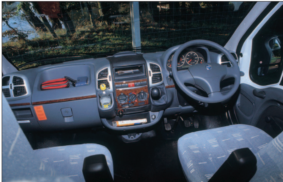
Latest Fiat cab has more car-like appearance with lots of storage and a much improved heater. Claims of executive saloon car levels of noise are debatable.
