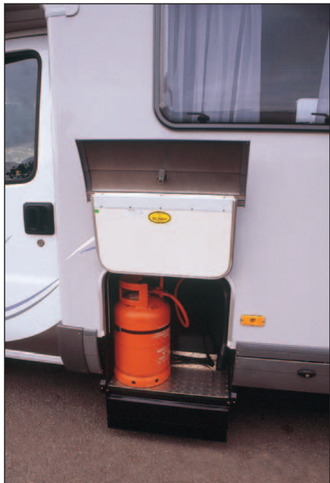
Gas locker accepts two 13kg cylinders.
