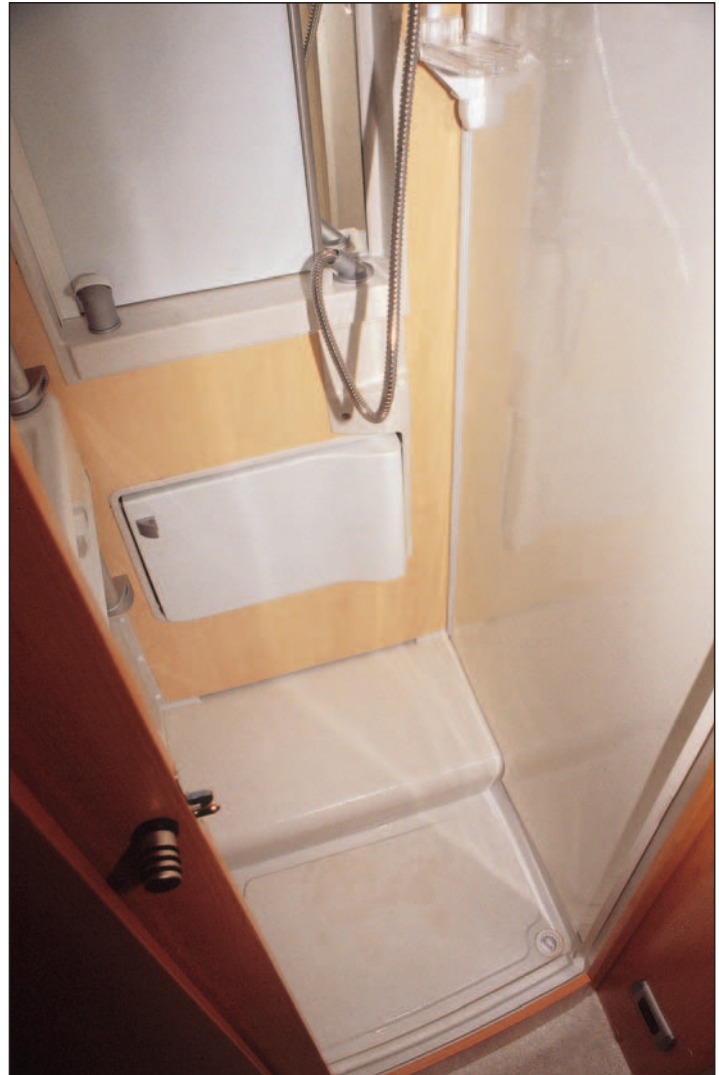
Combination tap clips on to shower rail and a sliding cover protects the mirror. Strong shower tray has two drain holes.
