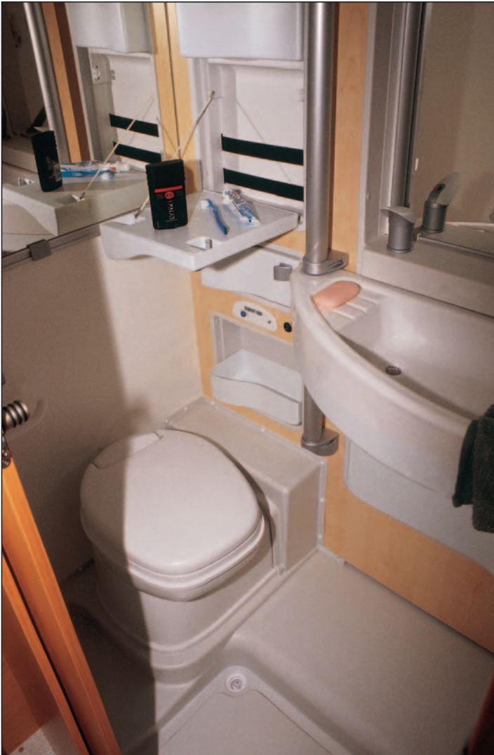
Excellent washroom has sliding door and elegant concealed lighting. Washbasin swings to the left on the vertical silver pole to create room for showering.
