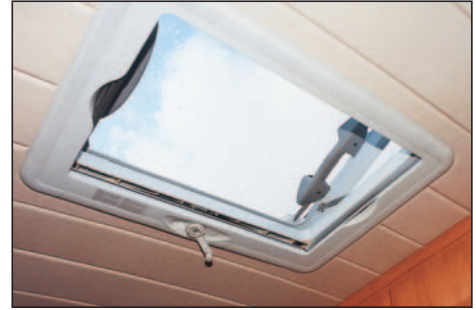
Heki 1 sunroof is standard on 'UK-spec' Hobby 750 - it tips every which way or winds up by rotary handle. Panelled ceiling is unusual.
