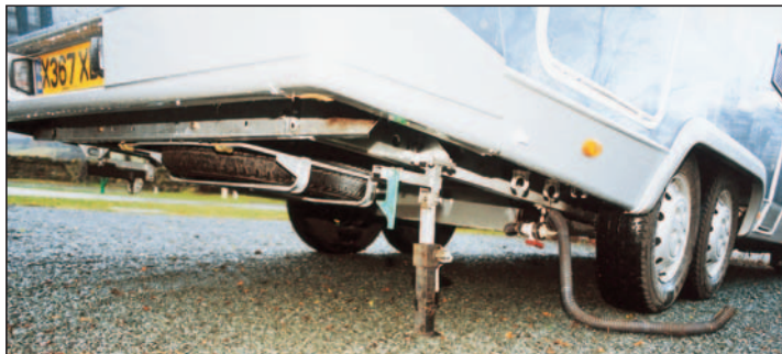
Simple-to-operate rear steadies and conveniently positioned spare wheel are pluses, grubby drain hose is a minus.
