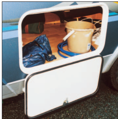
Large external hatch provides access to the heated under-bed locker, which can also be reached from inside the motorhome.
