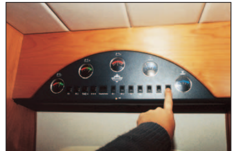
Comprehensive control panel with fresh and waste water level gauges. This is just above the caravan door.
