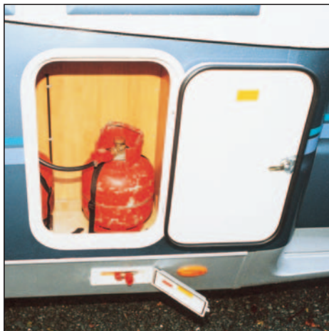
Gas locker can hold one 13kg and one 7kg cylinder. Gas point for barbecue can be seen below.
