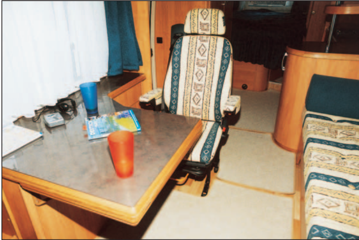
Third captain's chair in the rear is of a different style to the seats in the cab and comes with an integral three-point restraint.
