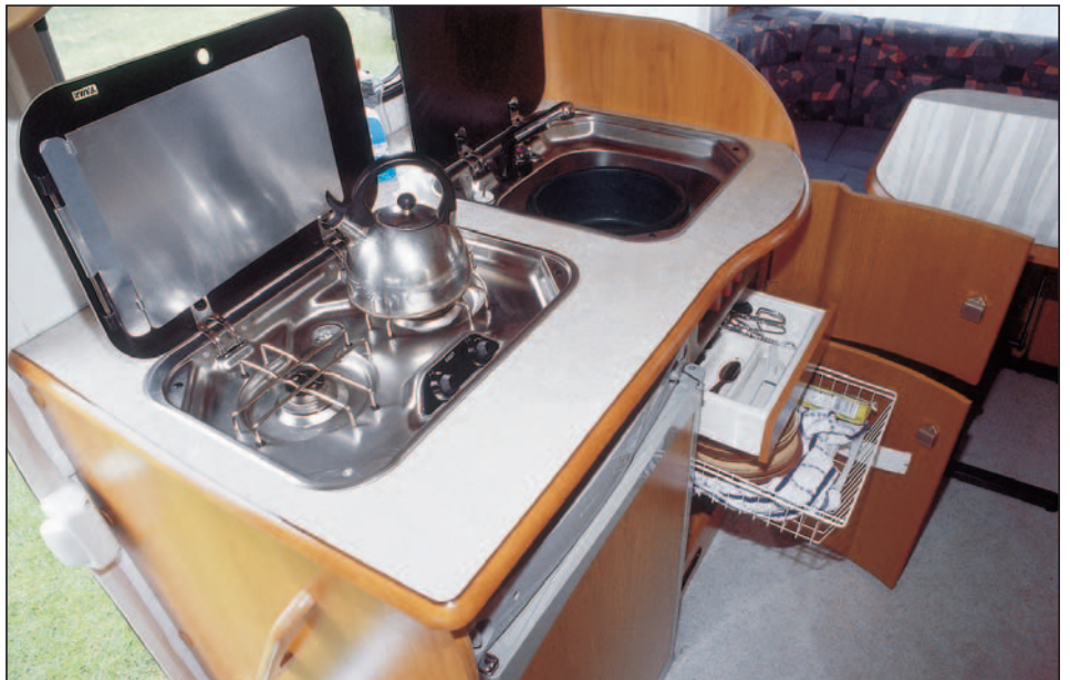
The galley makes do with a two-burner hob and drainer-less sink.
