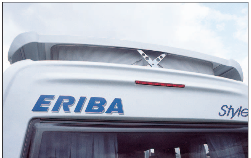
Eriba's pop-top (shown fully lifted) runs the full length of the roof, integrating with the bodywork when closed.
