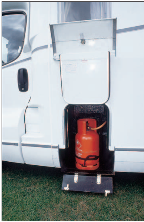
Seen here fitted with a 7kg cylinder, the gas locker has maximum capacity for only one 13kg cylinder.
