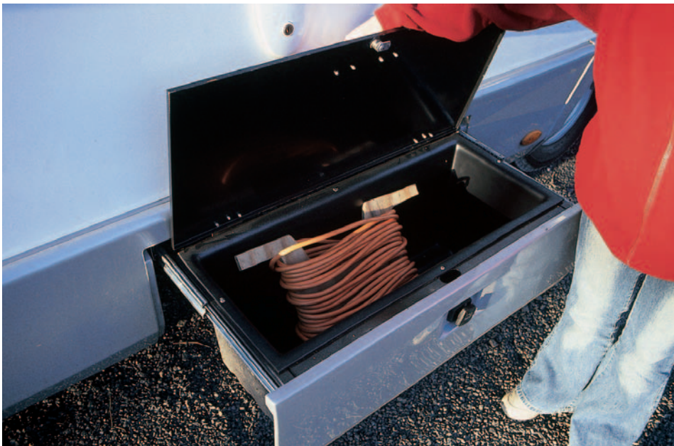
The lower skirt on the nearside has a sealed and well-made drawer for the wet or grotty stuff.
