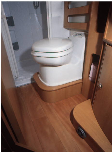
The main problem with the washroom is the lack of floor space due to these plinths below the toilet and sink.
