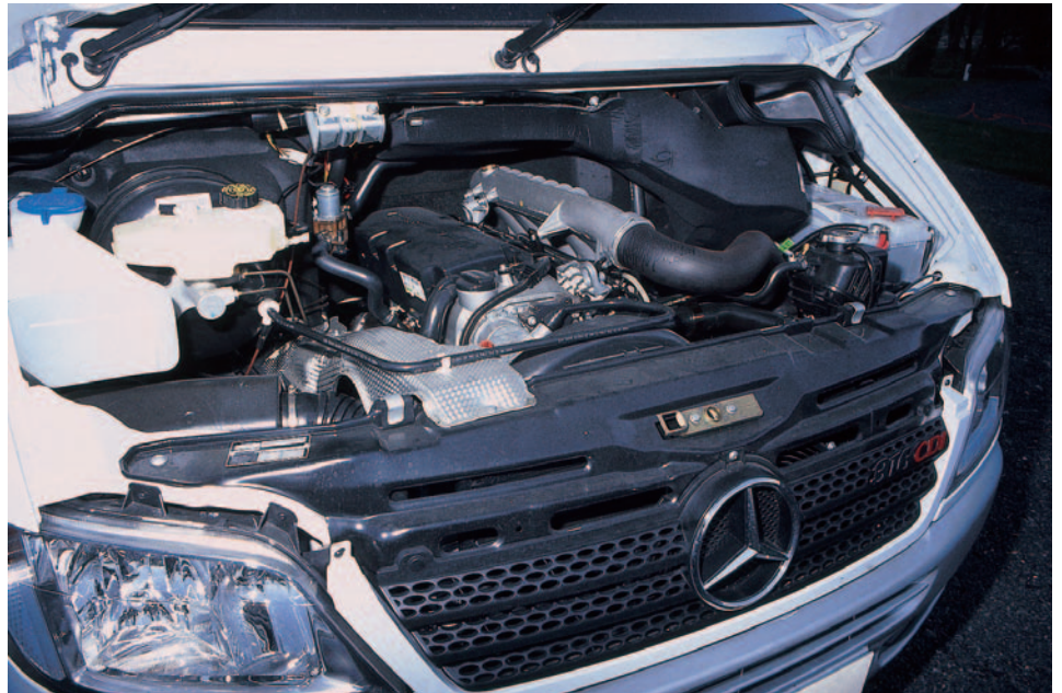
The five-cylinder Mercedes 2.7-litre engine. Fantastic.
