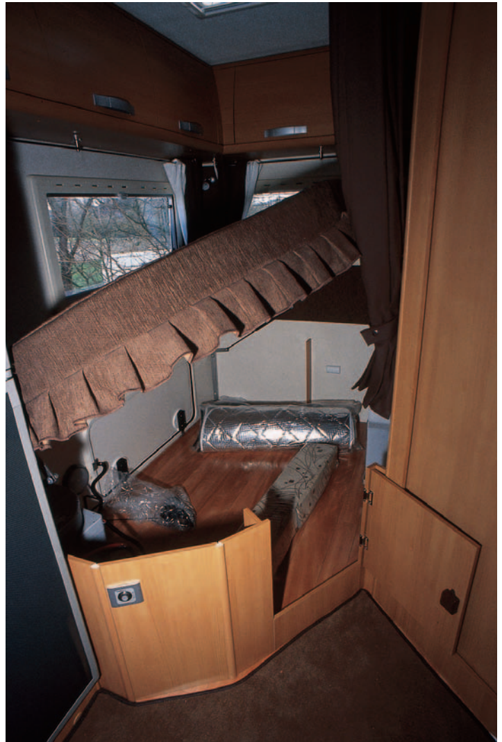
The fixed bed lifts easily on gas struts to allow access to the big locker underneath.
