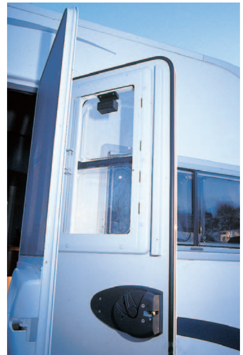
Entrance door with flyscreen and opening window. Unfortunately, you have to go outside to close the blind on the window.
