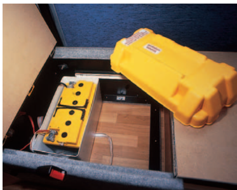
The auxiliary battery. Big, bright, and stored securely.
