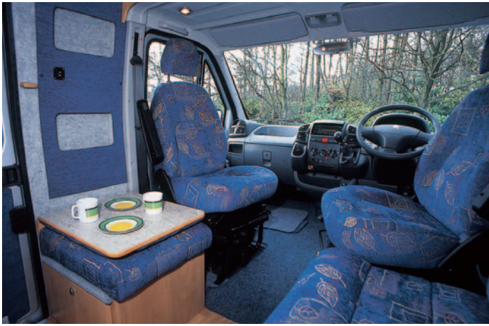
The backrest of the seat behind the passenger seat drops to create a very handy coffee table. What a simple but good idea.
