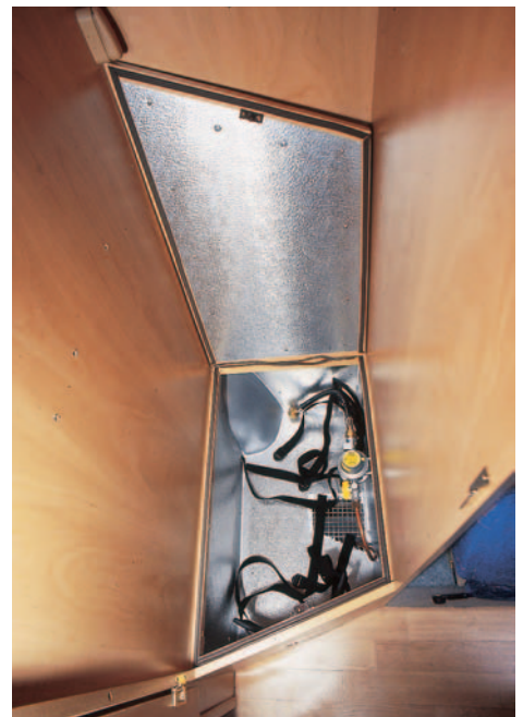
Gas locker - in the base of the wardrobe. Space efficient, but hard to get at come the inevitable cylinder change, and when the wardrobe is full. All part of the fun.
