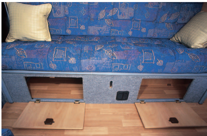
The only way to get at the under-sofa space is through these hatches. The only outlet for the space heater is here too, so don't expect a warm bathroom in the morning.
