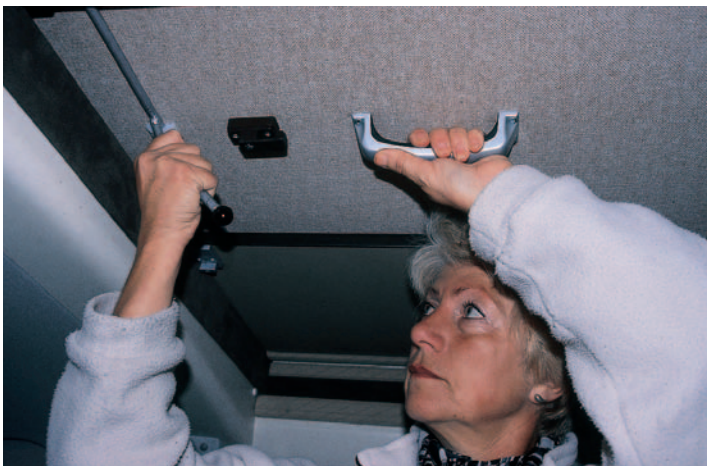
One of two levers that holds the roof down.
