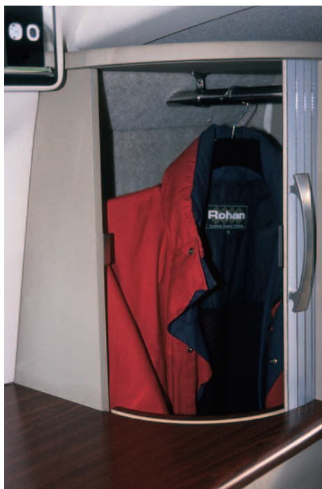
The slatted silver door enables quick access to the wardrobe. Strangely, the track for the slatted wardrobe door intruded into the interior space, when it could easily have been channelled along the side.
