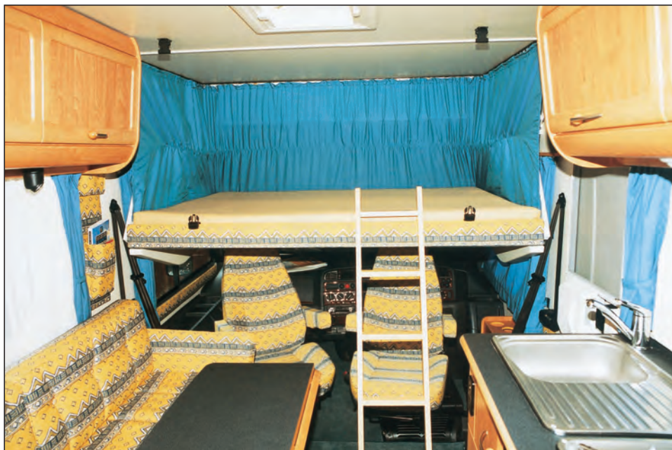
Drop-down cab bed has plenty of headroom thanks to flat roofline. Cab seats do not need to be moved before lowering bed.
