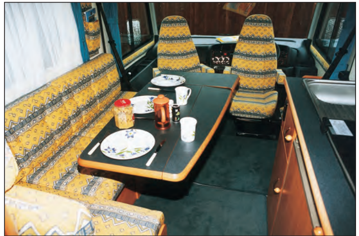
Extension panel at forward end of table makes room for banquets, but cab seats are lower, so all diners sit at the settee.
