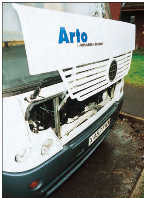
Arto bonnet lifts up almost vertically to provide typical A-class slot for engine access.
