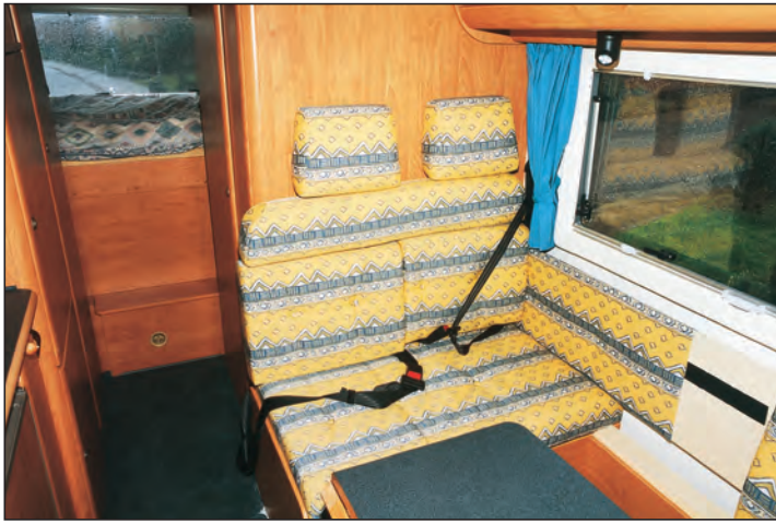
L-settee converts into double forward-facing seat for travel, but only one three-point belt is fitted (plus one lap belt).
