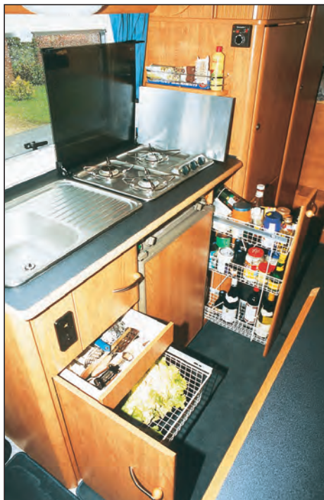
Kitchen storage includes large cutlery drawer, vegetable basket, waste bin, and slide-out pantry for tins and bottles.
