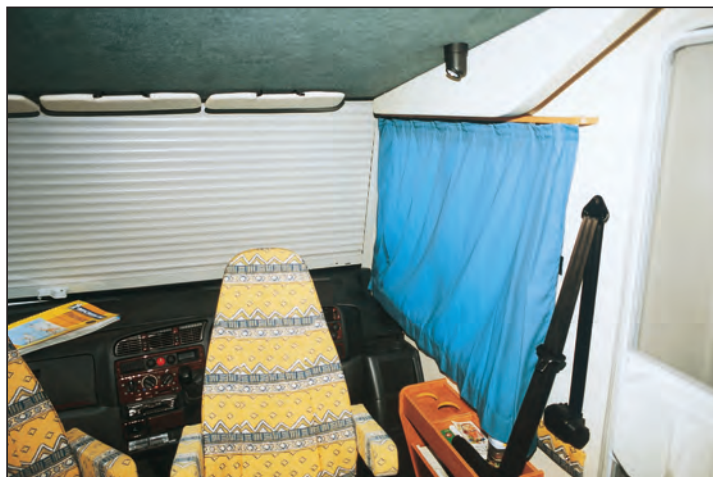
Windscreen has massive roller shutter blind but (double-glazed) cab side windows only have thin curtains.
