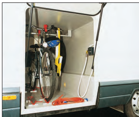
Rear garage is perfect for keeping a couple of bicycles clean and safe. External shower is situated here too.
