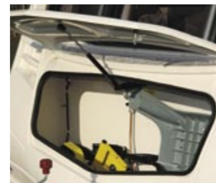
Front locker has a gas-filled strut to support the lid
