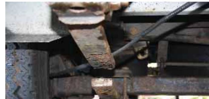
■ **Year 10 (2009)** – after fault-free period, a potentially dangerous event unexpectedly occurred at home on a cold February day. A rear suspension leaf-spring snapped (above). A flaw in the metal was clearly visible.
