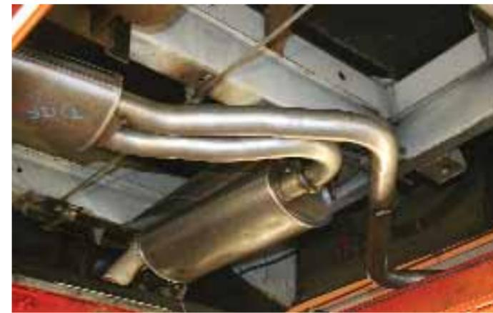
■ **Year 8 (2007)** – deep rusting on silencer boxes meant a new exhaust was required before the next MOT (above). Meanwhile, some of the original steel brake pipes needed replacing; good quality non-ferrous piping was fitted (right). Replacing other brake pipes almost became an annual job, probably hastened by winter driving on salted roads. In October, diesel exceeded £1 per litre.
