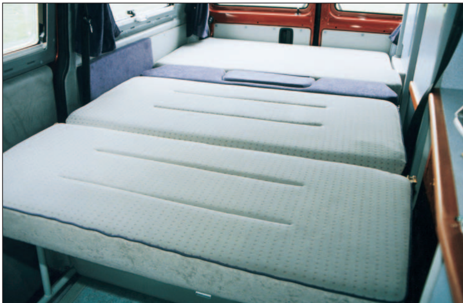
Lower double bed is easily made by sliding the rear seat forward and then flattening it out to join the boot area cushion.
