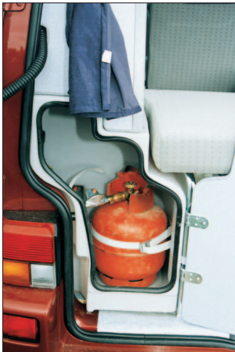
Gas locker will hold two 3.9kg butane cylinders or similar - more than most campers of this size.
