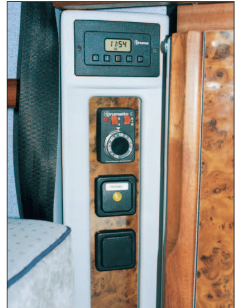
Panel next to kitchen cupboard is home to (from top to bottom) - timer for heating, temperature control for heating, switch for extra cooling fan for fridge, and 230V outlet.
