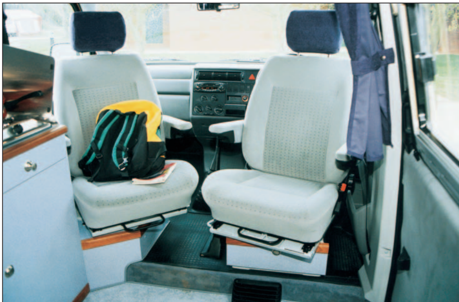
General view forward showing swivelled cab seats. Black rectangle on floor to the rear of driver's seat is the heater for rear passengers.
