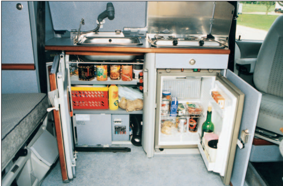
Kitchen ready for action. Cabinetwork was silent when on the move. Above the fridge is a cutlery drawer with moulded insert. See heater outlet bottom right of kitchen cupboard.
