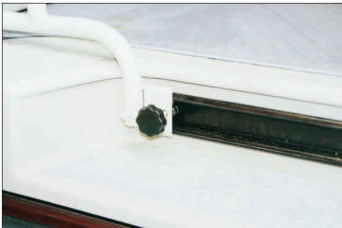
Seat tracking is cunningly hidden. Nearside is under cupboard run, and offside (pictured) is in the upstand of the entrance step well.
