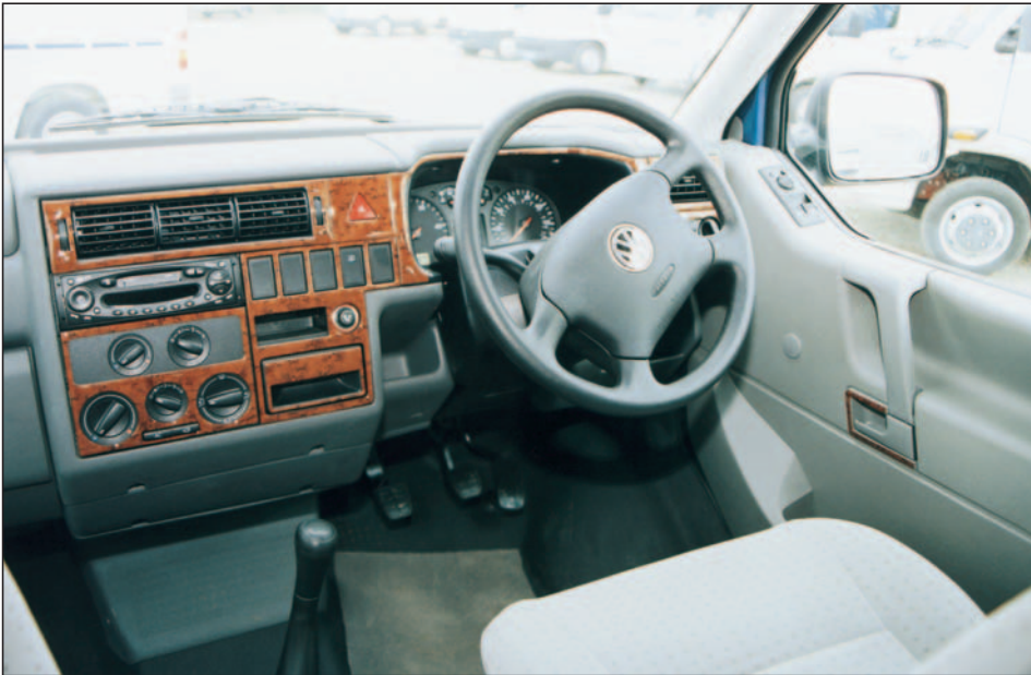
This is what the cab should have looked like. The wood trim hadn't been fitted to the test vehicle yet. See extra heater controls for rear heat exchanger (below radio).
