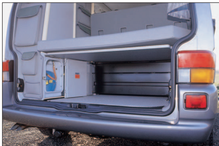
The gas locker is accessible from the boot. It holds one Campingaz 907 bottle - but with only the hob to power this should last a while.
