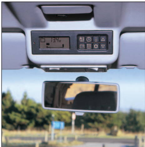
Centralised control panel allows timed control of the diesel-fired heater and regulation of the fridge temperature.
