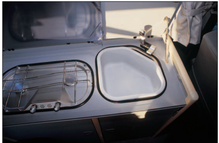
Two-burner hob has no grill or spark ignition. Sink is cold water only but has nifty multi-use fitted washing-up bowl.
