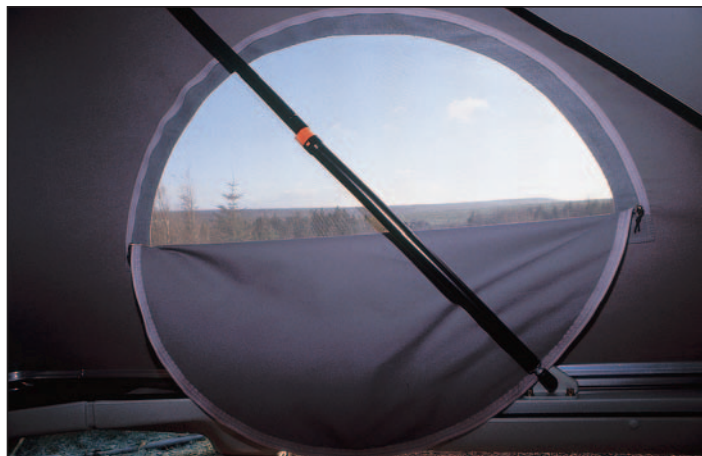
Rising roof has flyscreened vents with zipped covers.
