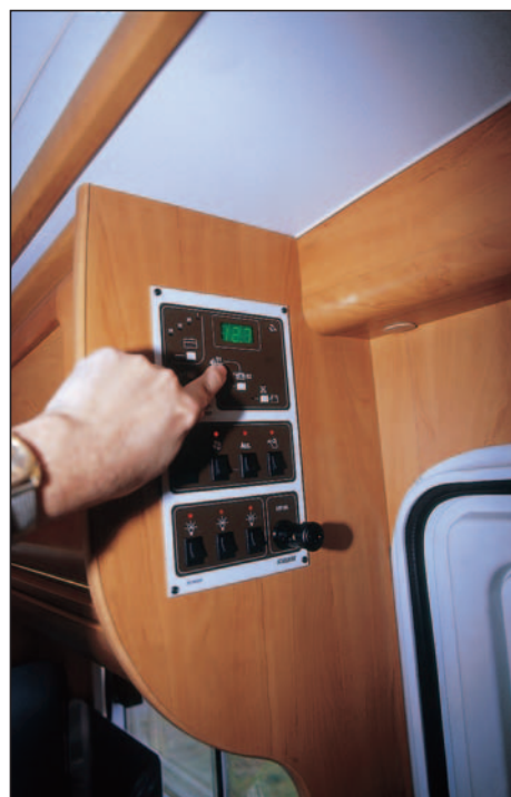
Easy-to-use control panel is adjacent to caravan door, has digital battery condition gauges, and fresh water level gauge, but waste tank just gets a full warning light.
