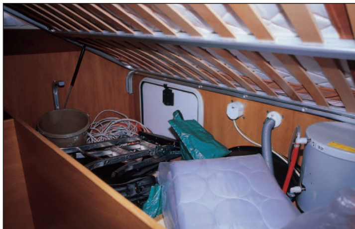
Vast amount of underbed storage (plus the boiler), but test vehicle had a problem with gas struts that raise the slatted bed base.
