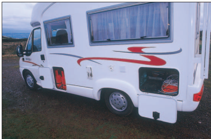
Nearside has gas locker, fresh water filler, mains hook-up, and access to underbed stowage.
