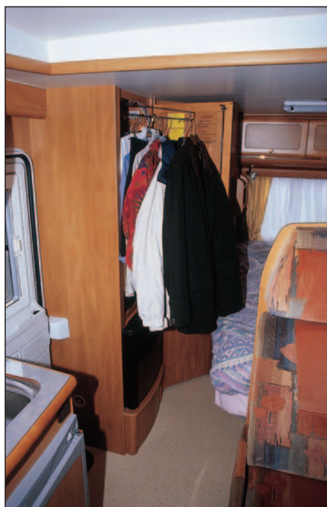
Wardrobe has front-to-rear hanging rail, which pulls out so you can reach rearmost garments. Plenty of room in here for two people's clothes.
