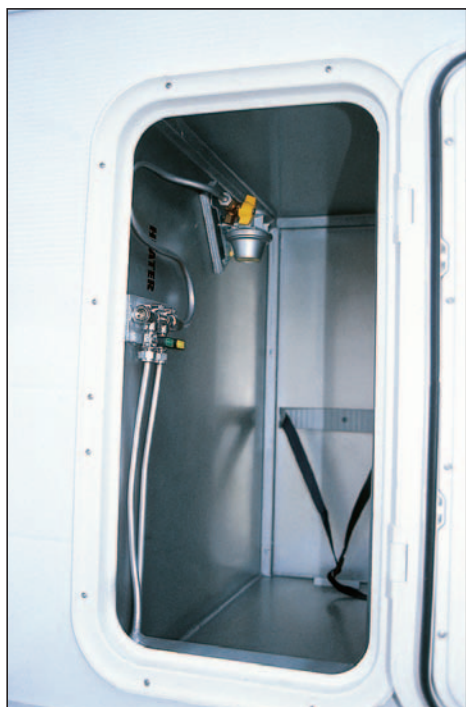
The gas locker has room for two 7kg cylinders, with the new-style fixed regulator.
