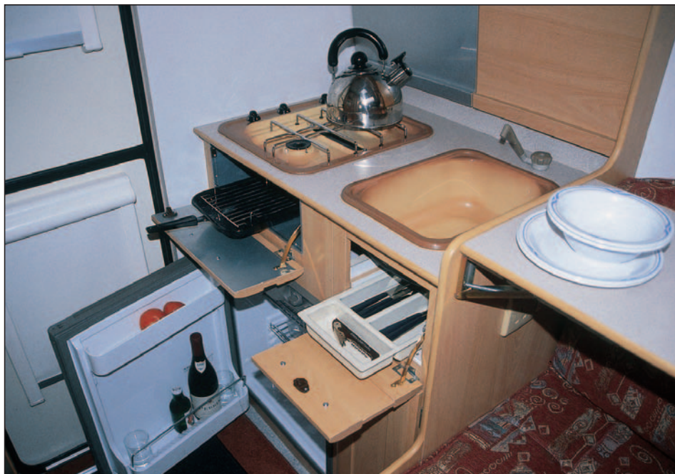
Two-burner hob, fridge, cutlery drawer; it's all there for the cook. No draining board but, if the hob cover is lowered, a tray could be used for that purpose.
