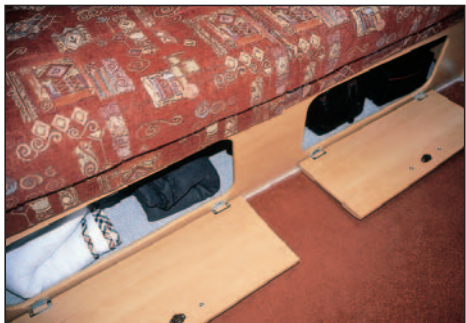
Storage under the settee can be accessed via these drop-down flaps.
