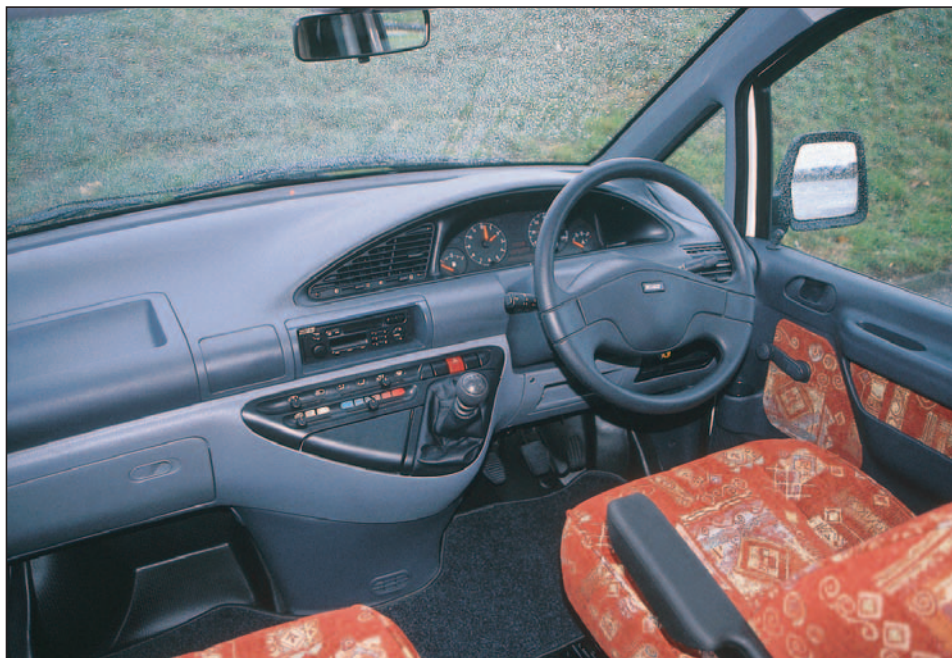
The Scudo cab, with its dash-mounted gearchange. A height adjustable steering wheel is a boon for different sizes of driver.
