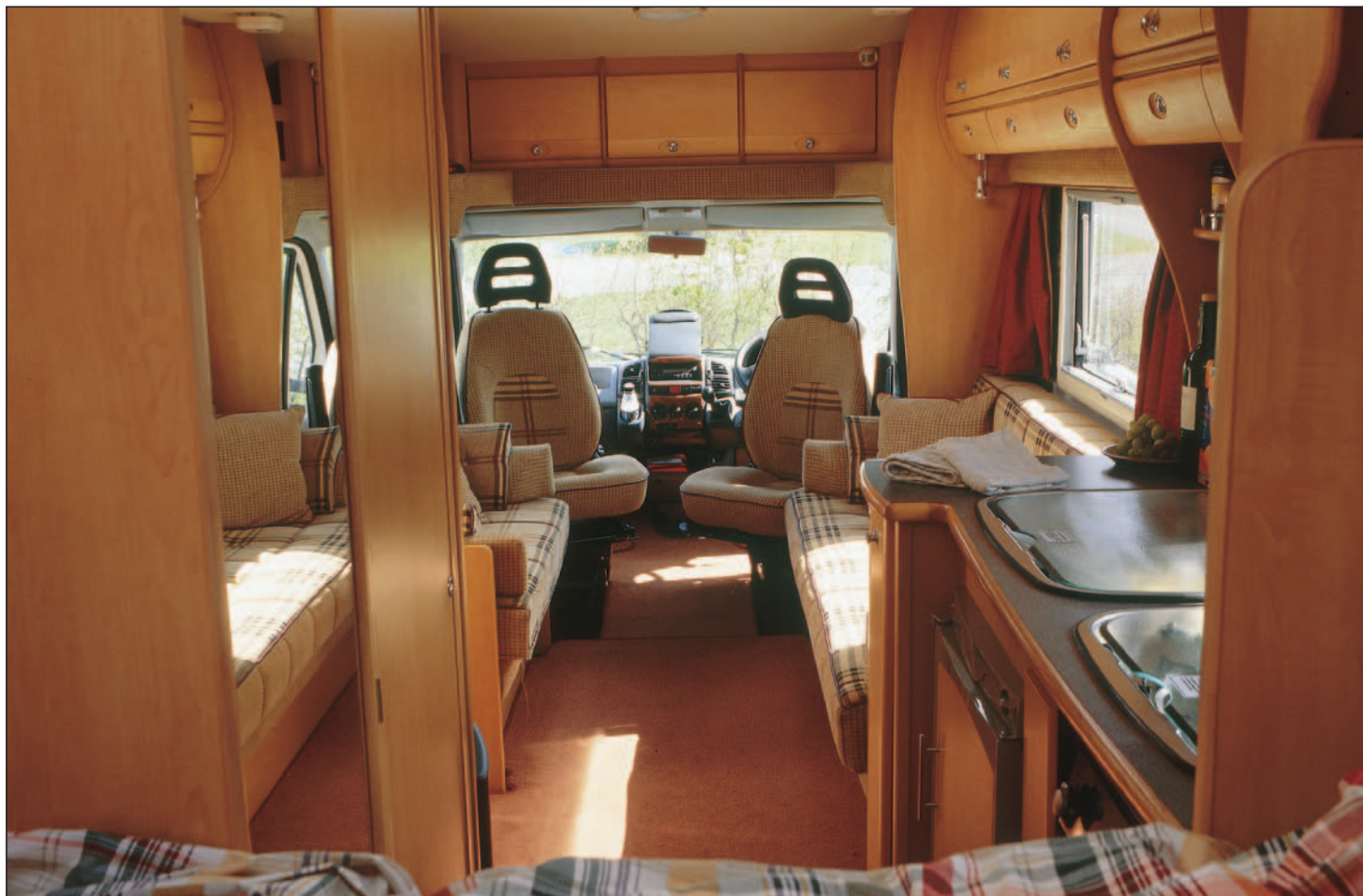
Looking forward from the fixed bed above the garage. The washroom (mirrored external wall) is on the nearside with the kitchen opposite. The lounge - with swivelled cab seats - is beyond.
