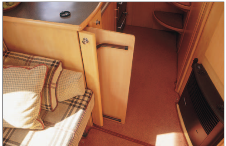
Excellent table storage was marred by a faulty catch, and the table came out to play after a few minutes on the road.
