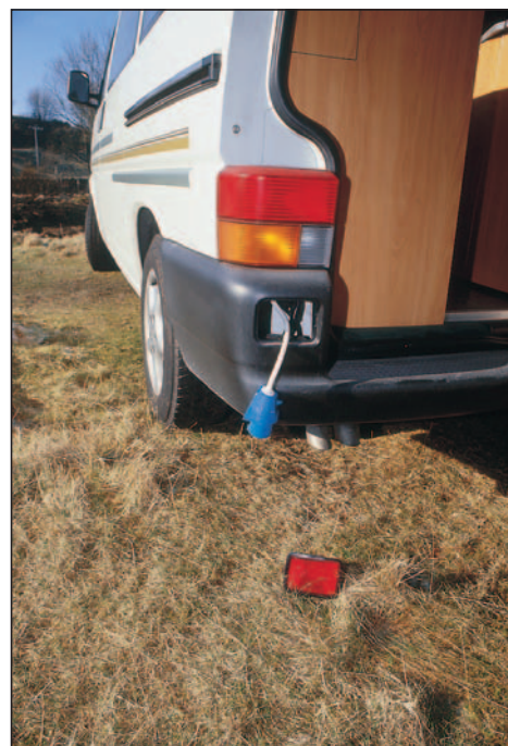
A dummy fog lamp is removed to reveal the hook-up socket.
