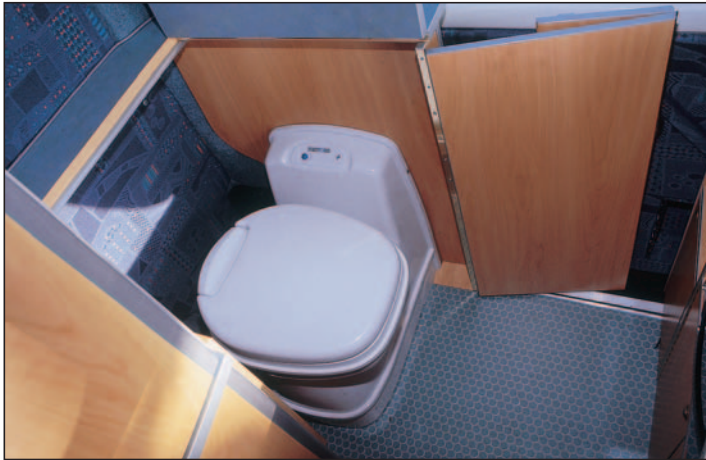
What appears to be a kitchen cupboard opens to reveal a full-sized, electric flush toilet.
