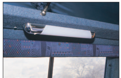
Stylish 12V fluorescent lamps are fitted throughout. I would have some spots as well, to soften the overall lighting effect.
