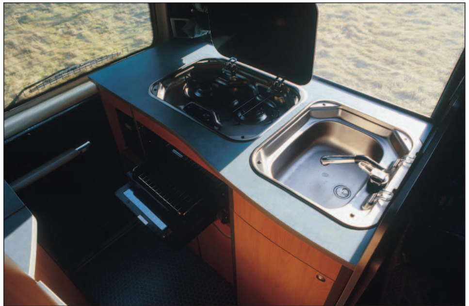
The main kitchen unit has matching hob and sink in stainless steel with grill unit below. The top of the toilet locker, opposite, is a handy place to put things while working.
