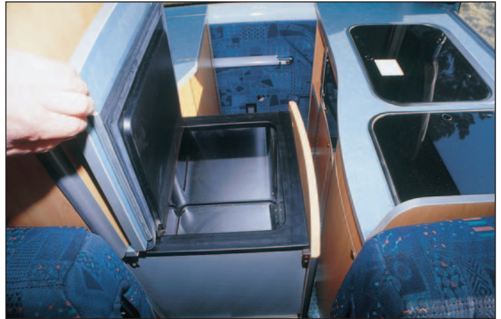
A slide-out unit reveals the top-loading fridge. It is awkward to use and a normal front-loading model would be far better.
