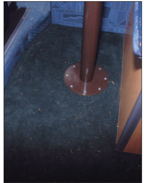
The location of the floor sockets for the table legs made it very difficult to get your feet under the table.
