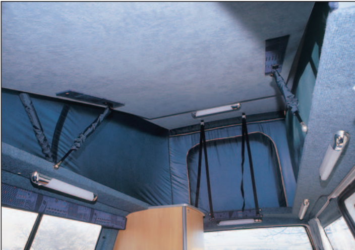
▲ The front-hinged rising roof creates generous headroom above the kitchen. The inner pair of struts supports the 'kids bed' in the roof.
