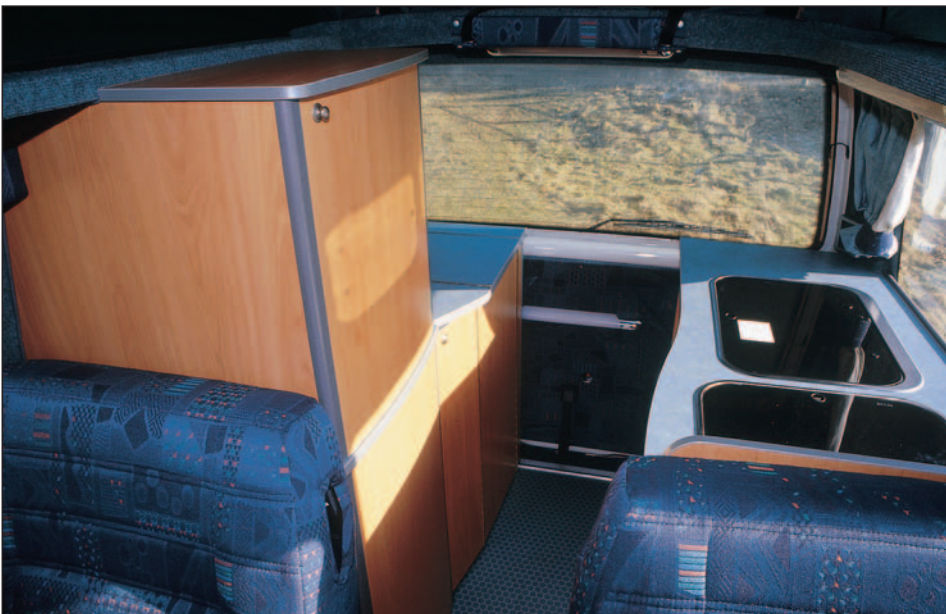
Rear furniture allows easy access day or night. The kitchen with hob and sink is on the right, while opposite is the wardrobe with pull-out fridge below and toilet cabinet beyond.
