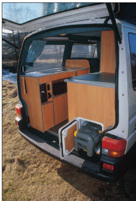
The toilet is serviced through the tailgate.
