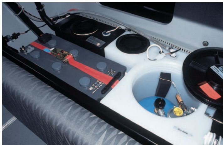
Under the kitchen unit are waste and fresh water tanks, massive leisure battery, and innovative gas cylinder storage.
