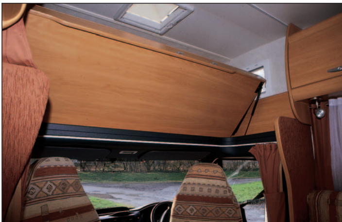
The caravan-side section lifts easily on gas struts to give more headroom in the lounge and ease access to the cab.
