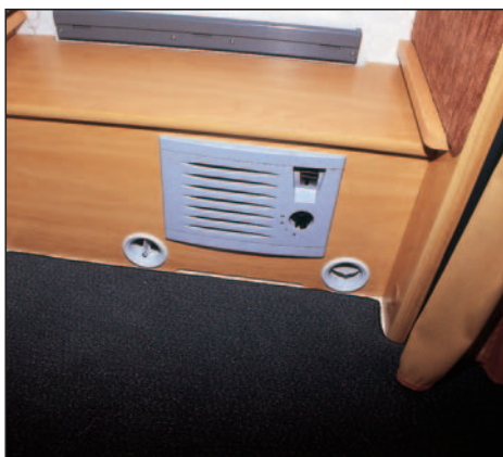
A rear-mounted heater matrix supplements the Ford cab heater to keep rear passengers toasty.
