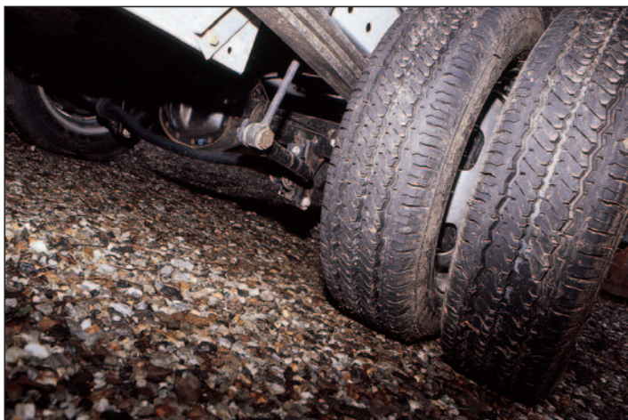
The driven rear axle, with twin wheels, gives good handling and excellent traction and payload.
