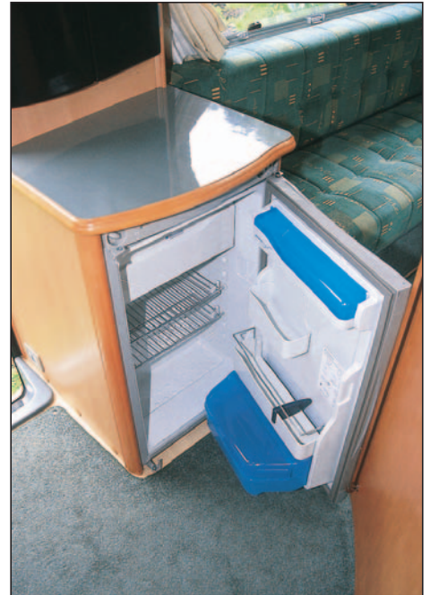
The Dometic three-way fridge has sufficient room to cater for all needs. The shiny work surface is attractive, but (judging by the score marks in it already) may not be a practical long-term proposition.
