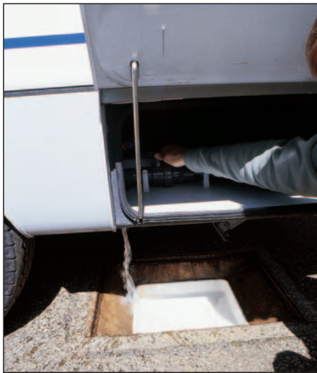
Draining waste water is simple with an easy-to-use valve located inside a skirt locker.
