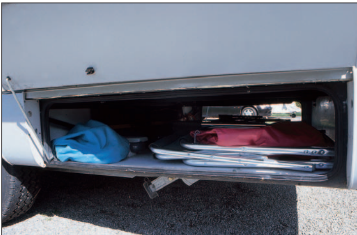
The double floor construction provides a home for tanks and pipes, plus storage compartments for all your flat stuff.
